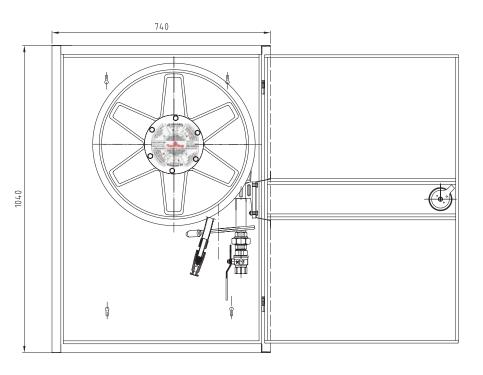
Hose reel arm comes with wall mounting base plate that can easily be installed to the bracket inside the cabinet using nuts provided.
